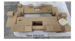
> Orientation for detached pad block to pad block and pad block to pad base.
